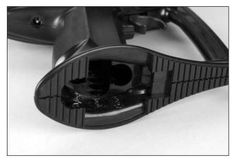
3. Install the AA batteries into the transmitter. Be aware of the proper polarity when inserting the batteries.
