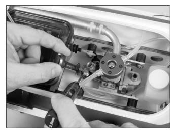
4. Carefully pull the ferrule away from the stuffing tube. You will need to pull at an angle to clear the aluminum strut.
