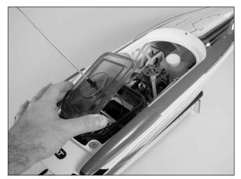
3. Remove the dry cell battery holder from the radio box. Install four AA alkaline batteries as shown with respect to polarity.
