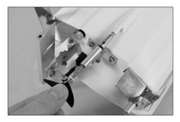
3. Insert a hex driver into the hole located on the flywheel to lock the crankshaft in place. Then use a 10mm wrench to loosen the collet nut.
