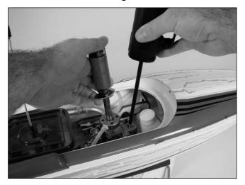
**Note**: Stop operation immediately if the engine enters a hydro-locked condition, as serious engine damage may occur. Remove the glow plug, invert the boat and operate the starter to remove raw fuel before resuming operation.
