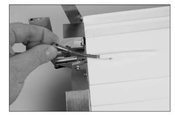
5. Clean any residue off of the flexshaft and liberally lubricate the entire length of the flex shaft with silicone cable grease as shown.
