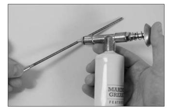
6. Carefully re-install the flex shaft and nylon bushing, making certain that you correctly tighten the collet nut. Next, re-install the drive shaft and propeller and tighten the setscrew on the flat of the drive shaft. Use threadlocking compound to secure the setscrew.
